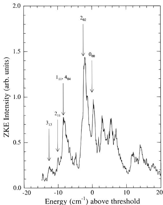
**Figure 4.** ZKE spectrum near the threshold, showing appearance of different rotational levels of NO<sub>2</sub>.
