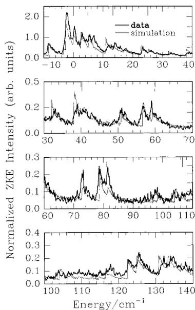
**Figure 5.** Comparison of phase space theory prediction for a maximum impact parameter of  $l_{\max} = 5\hbar$  (light line) and the experimental data (heavy line). The long ticks on the top axis of the top three panels give expected positions for the opening of the lower spin-orbit NO rotational channels starting from the ground rotational level of NO<sub>2</sub>.
