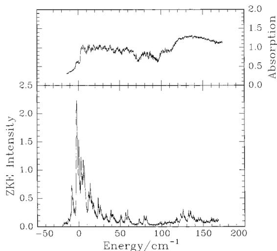
**Figure 3.** Zero Kinetic Energy spectrum of O(<sup>3</sup>P<sub>2</sub>) from NO<sub>2</sub> dissociation.
